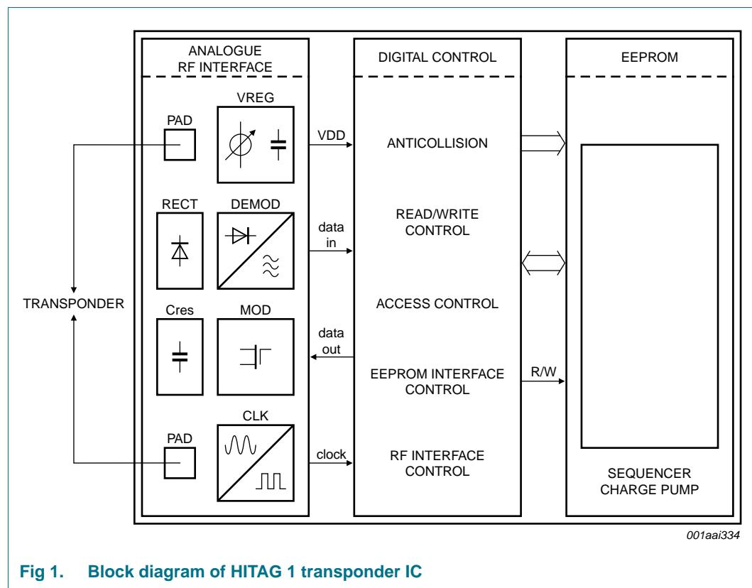
Fig 1. Block diagram of HITAG 1 transponder IC
