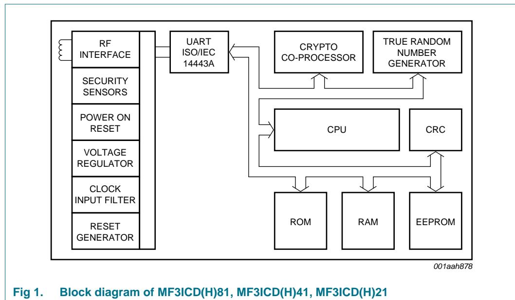
**Fig 1.** Block diagram of MF3ICD(H)81, MF3ICD(H)41, MF3ICD(H)21
